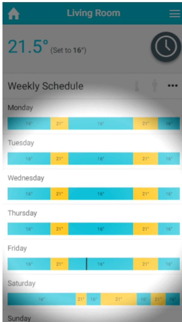
The main difference between Timer mode in Radiator, Underfloor heating or Hot Water Temperature zones compared with On/Off zones is that you can set a temperature for these types of zone. In On/Off zones you can only set periods where the heating is on or off.
